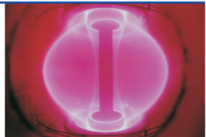
In a tokamak the plasma is held in a doughnut-shaped vessel. Using special coils, a magnetic field is generated, which causes the plasma particles to run around in spirals, without touching the wall of the chamber. (Courtesy: EFDA).
