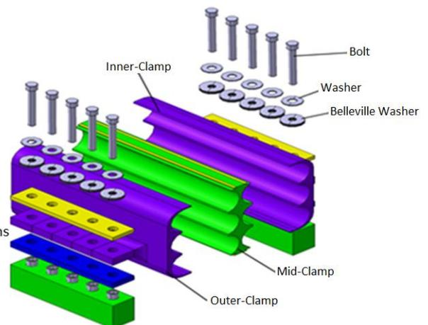
Figure 3: the explosion view of the bracket
