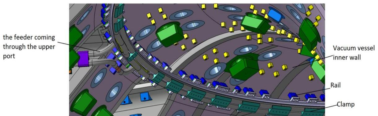
Figure 6: Integration of the Upper VS coil
