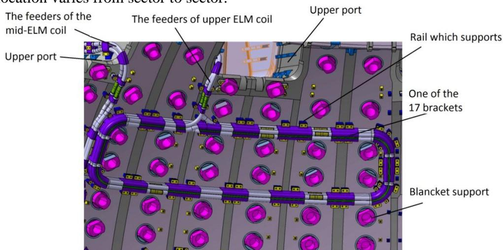
Figure 5: Example: Upper ELM coil installed on the VV wall
