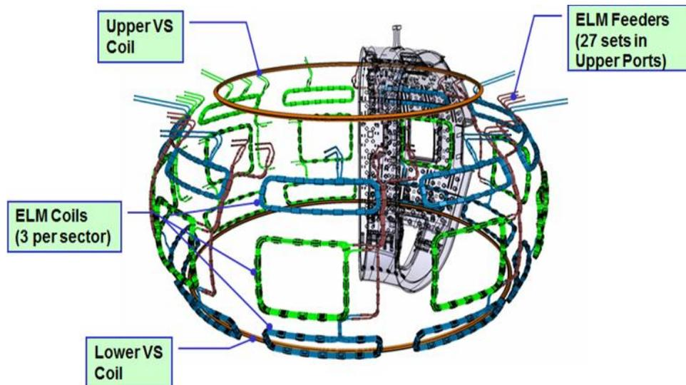
Figure 1: Overview of the IVCs inside the machine
