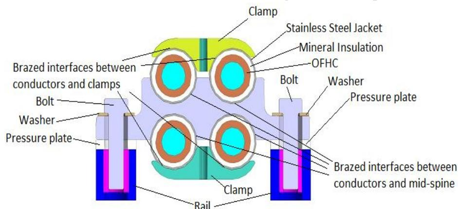
Figure 4: Cross section of VS coil with clamps and mid-spine
