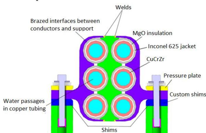
Figure 2: Cross-section of ELM coil with bracket
