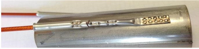
Figure 5-2: SC to HV wire connection
