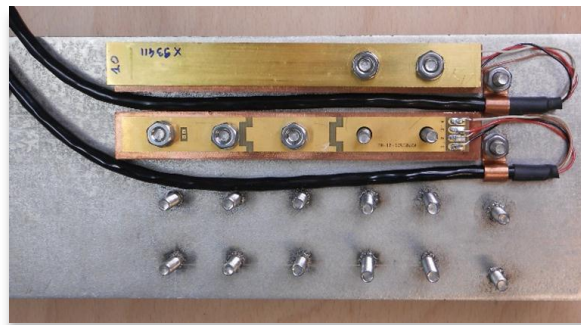
Figure 5-44: Thermometric blocks mounted on welded studs, with and without thermal shield.
