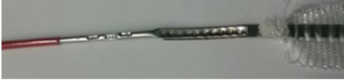
Figure 5-3: CWT to HV wire connection
