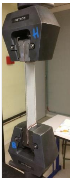
Figure 5-9: Illustration of CWT type 2 tensile test.
