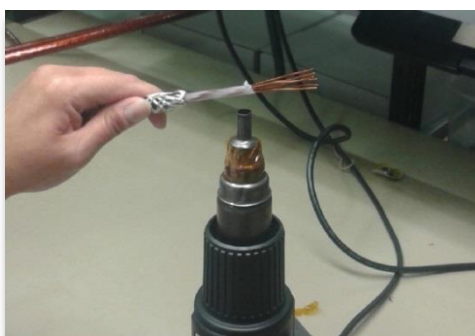
Figure 5-19: Illustration of HV vacuum cable spool and picture of the stripping test
