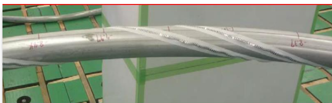
Figure 5-8: Illustration of CWT type 1 wrapping on a TF conductor.
