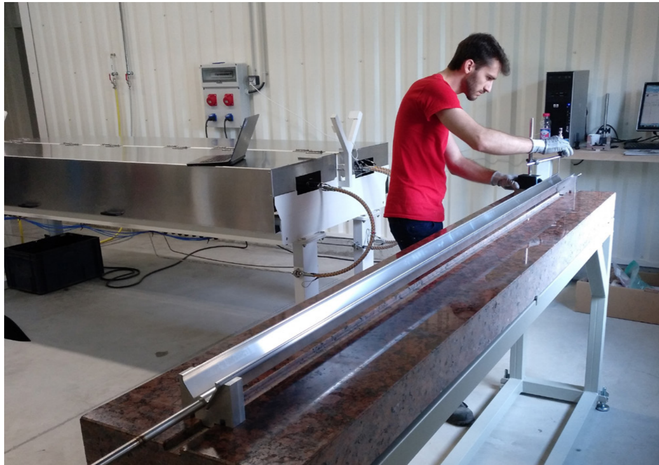
A technician performing a metrological survey on a V-shaped thermal radiation shield, May 2019 © Ravanat
