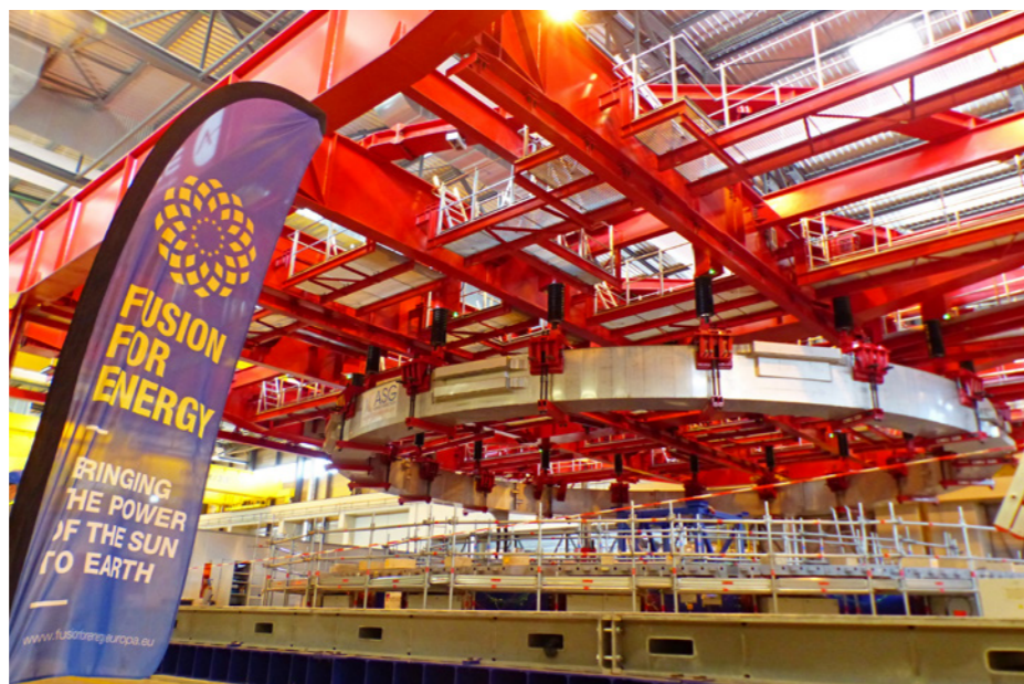
PF coil 5 lifted with clamps before cold tests start, F4E PF coils factory, ITER site, Cadarache © F4E
