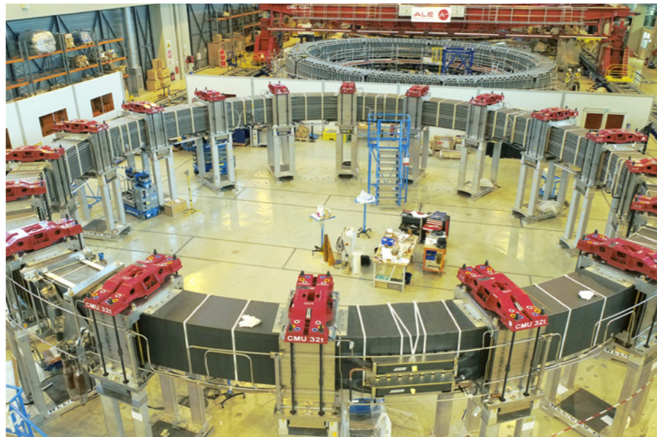
PF 5 undergoing dimensional inspection using laser technology. In the back, PF2 assembled inside the impregnation station, Cadarache, November 2020 © EJF Riche/ITER Organization
