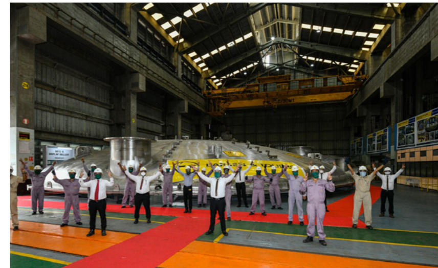
650-ton lid of Cryostat completed, it's the fourth section of the component in order of assembly after the base, the lower cylinder and the upper cylinder.
