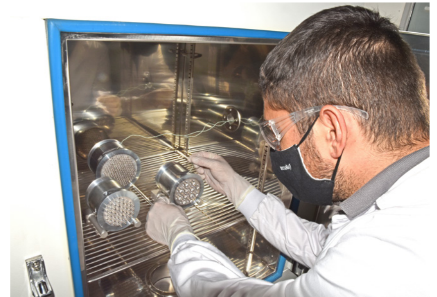
Feedthrough prototypes placed in an oven to simulate the thermal stress caused by 500 baking cycles. The thin cables read the temperature inside the prototypes. F4E signed a contract with IDOM for the development of the prototypes. The tests were performed by Tecnalía. ©Tecnalía
