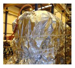
Helium leak test of 20 m<sup>3</sup> tank
