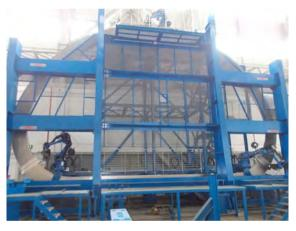
The three big sectors of the Radial Plate are being welded in the welding frame at the SIMIC site (Courtesy of SIMIC)
