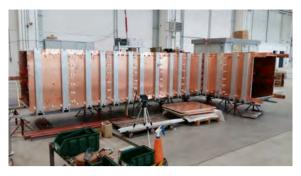
The SPIDER Transmission Line during the assembly at the NBTF
