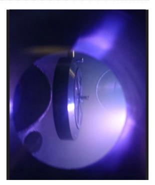
Mirrors being cleaned by RF plasma
