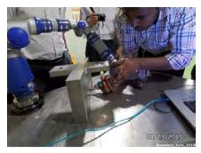
A vacuum vessel shielding block inspection
