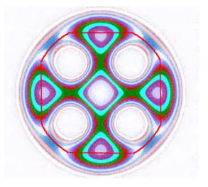
Calculated space charge potential profile for the quad-core MI cable
