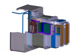
Two European Test Blanket Modules and their radiation shields installed in the ITER Port Extension #16 (IDOM)
