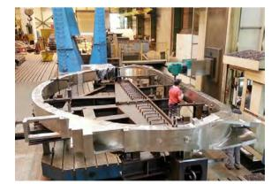
Final machining of coil no. 10 (November 2015) (Courtesy ALSTOM/CEA).
