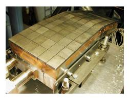
First Wall qualification semi-prototype manufactured by ARE-VA and tested at TSEFEY-M
