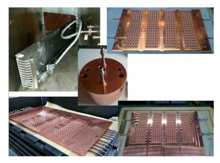
The SPIDER beam source components ready for assembly
