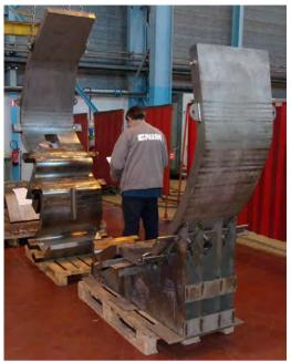
Cassette body prototype under fabrication at CNIM
