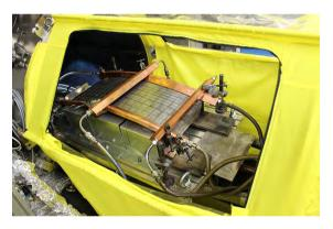
First Wall semi-prototype manufactured by the Consortium IBERDROLA/Amec FW/Leading and tested at JUDITH-2
