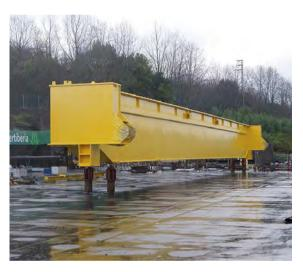
Crane 750 t first girder, stored at the factory location before assembly and squaring
