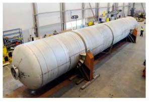
LHe tank inner vessel helium leak test
