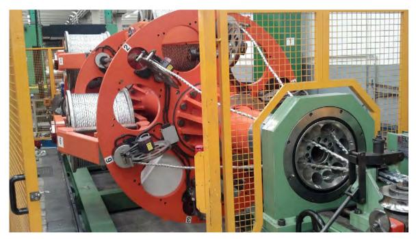
Fifth and last stage of Toroidal Field conductor cable fabrication at Tratos/ICAS
