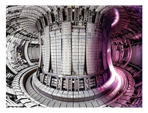
Inside JET's doughnutshaped vacuum vessel, plasmas (overlaid image) are confined using magnetic fields and heating to enormous temperatures to create fusion reactions (courtesy of EUROfusion)
