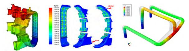
Vessel sector 5 displacements (left) during a VDEII, its nuclear heat for 500 MW scenario (centre) and MECOS piping systems under benchmark analysis: example of computed eigenmode
