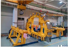
Coil 1 – welding of casing after coil insertion (September 2015) (Courtesy ASG/ENEA).
