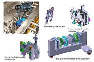
Snapshots illustrating the NBRHS pipe tooling design
