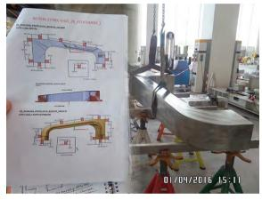
Large forging of the vacuum vessel
