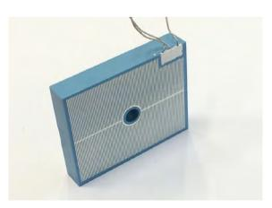
One of the LTCC sensor prototypes manufactured by Via Electronic GmbH
