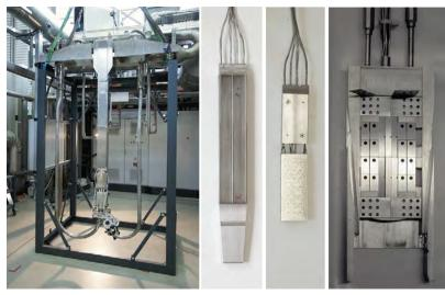
Fabricated prototype items: Left: The HFTM double compartment prototype during installation in HELOKA-LP; Middle: a completed rig and a capsule with upper reflector; Right: The specimen stack in a so-called assembly tray before insertion into the capsule
