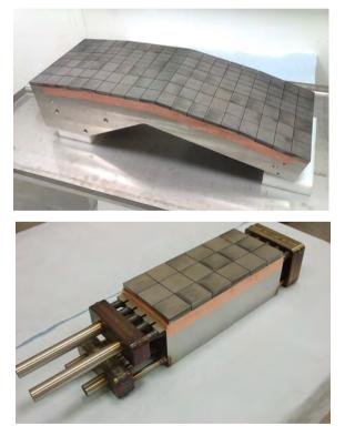
First Wall semi-prototype (left) and general R&D mock-up manufactured by the Consortium Iberdrola/Amec FW/Leading
