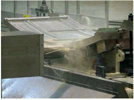
Machining activity on large forging
