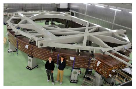
Series DPs, stacked together to form the first ITER TF coil Winding Pack in ASG, La Spezia (Courtesy of ASG)
