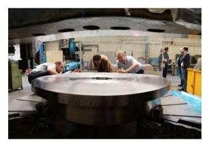
The pump plug of the pre-production cryopump in manufacturing
