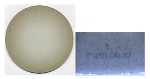
One of the qualified disks (left) and close-up of ID mark of the disk (right) – Diamond Materials (OPE 561).
