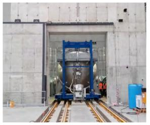
The SPIDER vacuum vessel inside the bio-shielding
