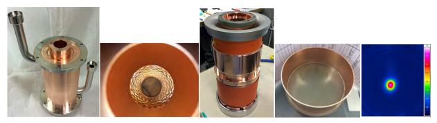
Subassemblies of the 1MW CW gyrotron prototype: the beam tunnel external and internal sides, electron gun, collector, and the output diamond window; and the IR image of the output window from the short pulse gyrotron showing a high Gaussian mode content of the output microwave beam (~98%).
