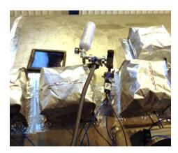
Helium leak test of 100 m<sup>3</sup> tank
