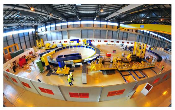
PF 2-5 Winding Machine installation in the PF Building at the Cadarache site
