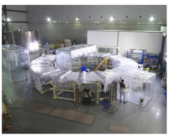
Working on the terminations of one Double Pancake of Poloidal Field coil 6, ASIPP, China
