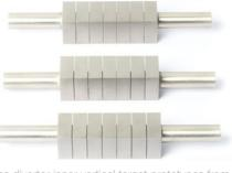
The divertor inner vertical target prototypes from ATMOSTAT-ALCEN
