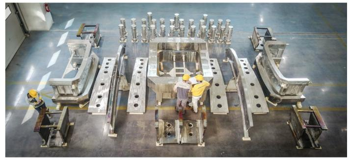
each of the five sectors is at a different stage Notable in terms of qualification, is that in part due to the past experience, CNIM was able to qualify its welding techniques according to the nuclear code in less than two months. a record in comparison to earlier welding gualification times.
