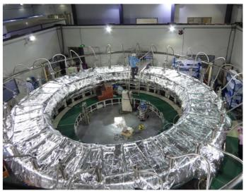
Performing impregnation on a Double Pancake mock-up of Poloidal Field coil 6, ASIPP, China
