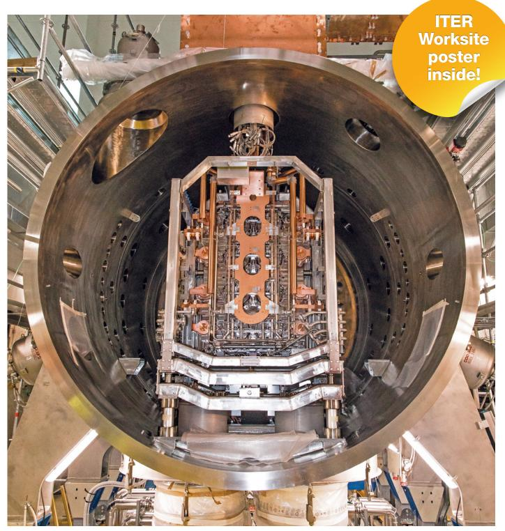
SPIDER beam source installed in the vacuum vessel, ITER Neutral Beam Test Facility, Padua, Italy © RFX
