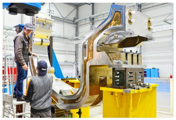
of the 54 ITER Divertor Cassettes, F4E in collaboration with industry had to develop real-size cassette prototypes to demonstrate the feasibility of their fabrication. For this reason, Europe developed a procurement to get involved in order to check whether minimum cost.
