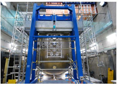
Getting ready to lock the SPIDER beam source in its vessel, ITER Neutral Beam Test Facility, Consorzio RFX, Padua, Italy
