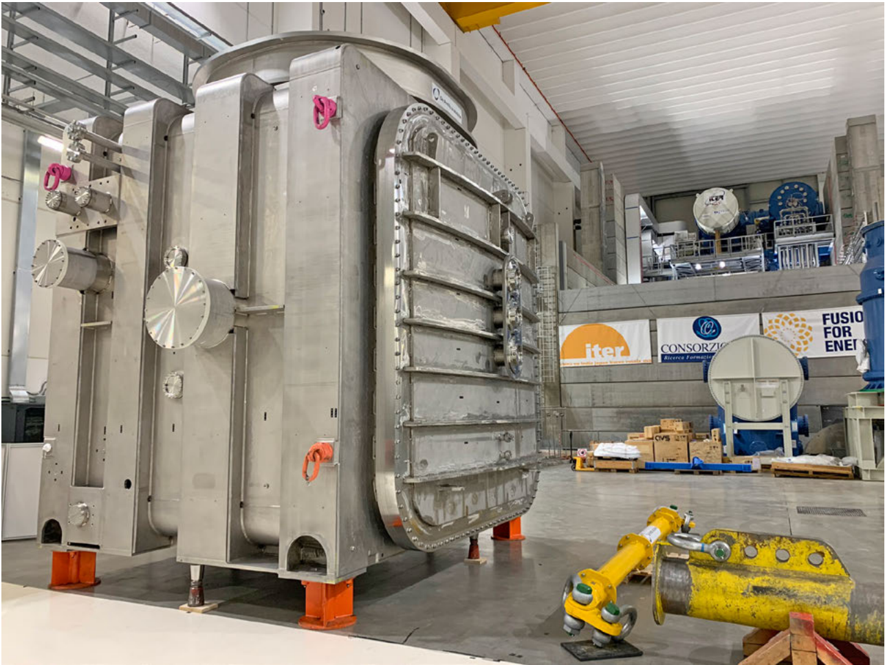
MITICA beam source vacuum vessel delivered to ITER Neutral Beam Test Facility, Consorzio RFX, Padua, Italy. The component has been manufactured by De Pretto Industrie and financed by F4E.
