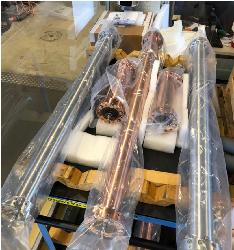
Short waveguide mock-ups (CuCrZr) and three 1.2 m waveguide mock-ups, in Stainless Steel, CuCrZr and Aluminium, manufactured by TBB under F4E contract.
