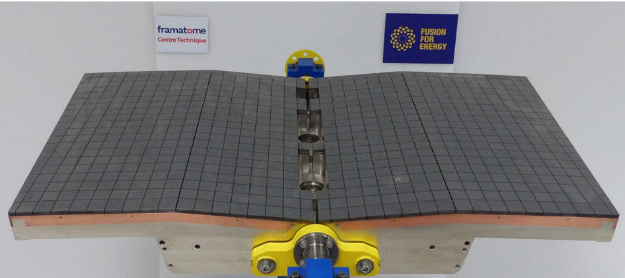
ITER first wall panel full-scale prototype manufactured by Framatome, financed by F4E.
