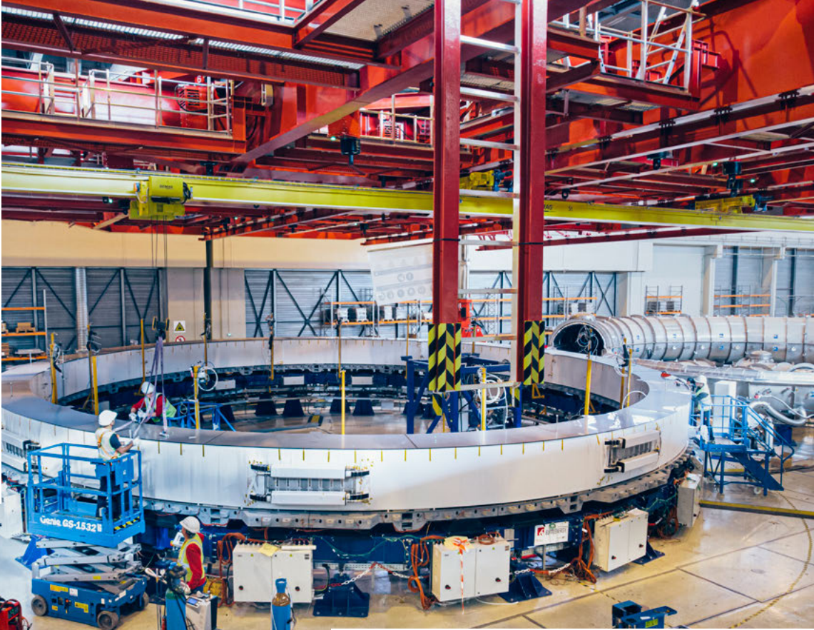
Poloidal Field coil 5 positioned to the impregnation table, in the PF coils factory, November 2019, Cadarache, France © F4E
