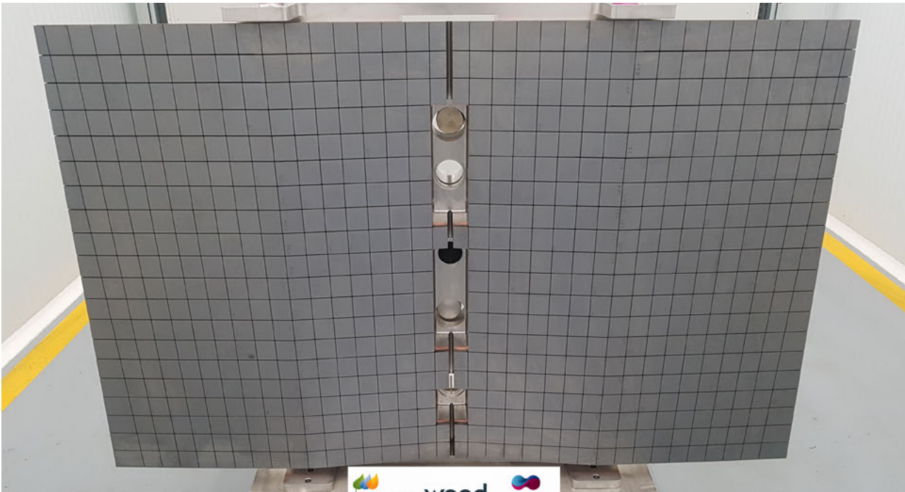
ITER first wall panel full scale prototype manufactured by Iberdrola, Leading and Wood, financed by F4E.
