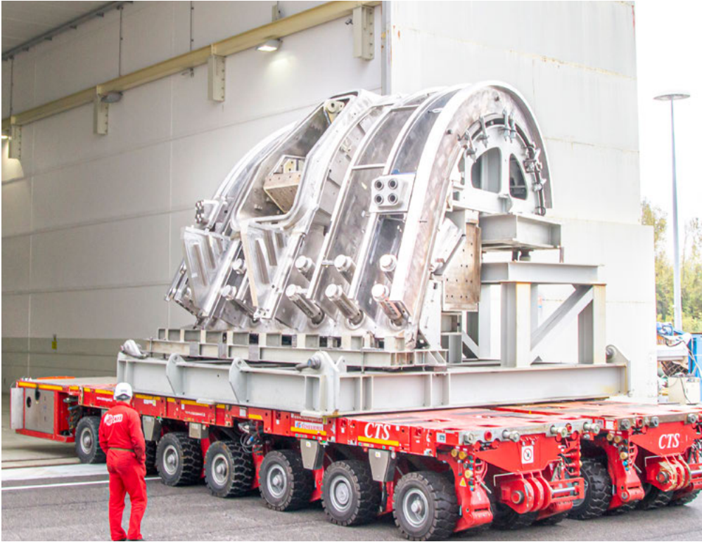
Lower segment of sector 5 of the ITER Vacuum Vessel loaded on a trailer to go through radiographic tests. Works performed in Mangiarotti, located in Monfalcone, Italy.
