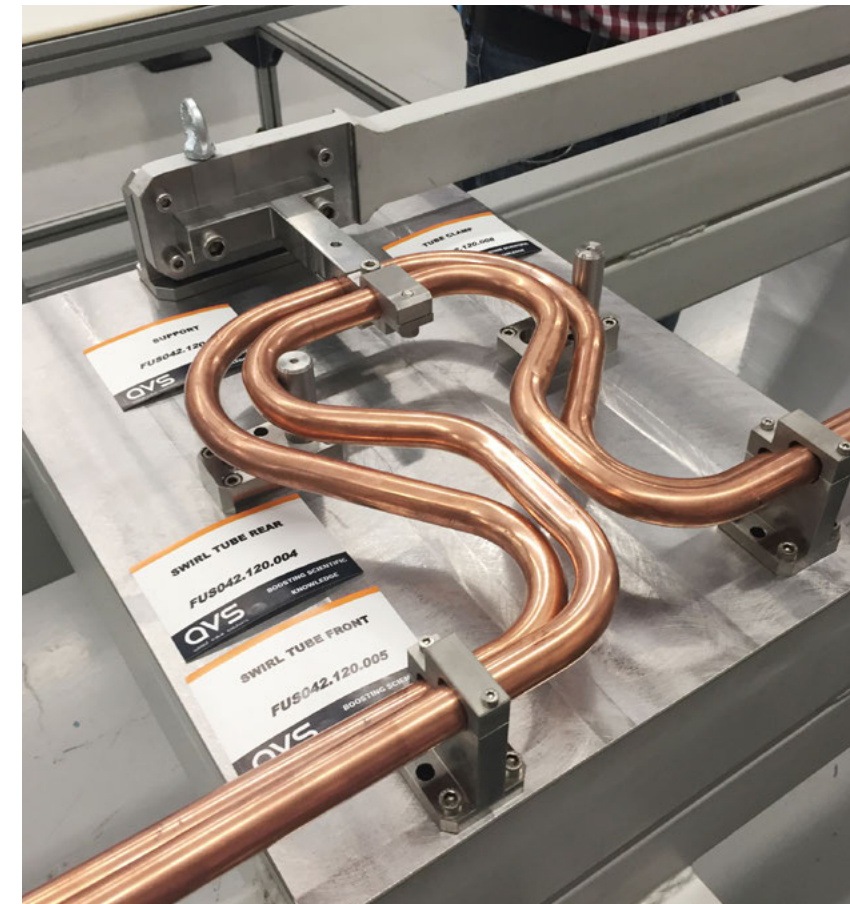
Swirl tube element prototype produced by the AVS-TECNALIA consortium
