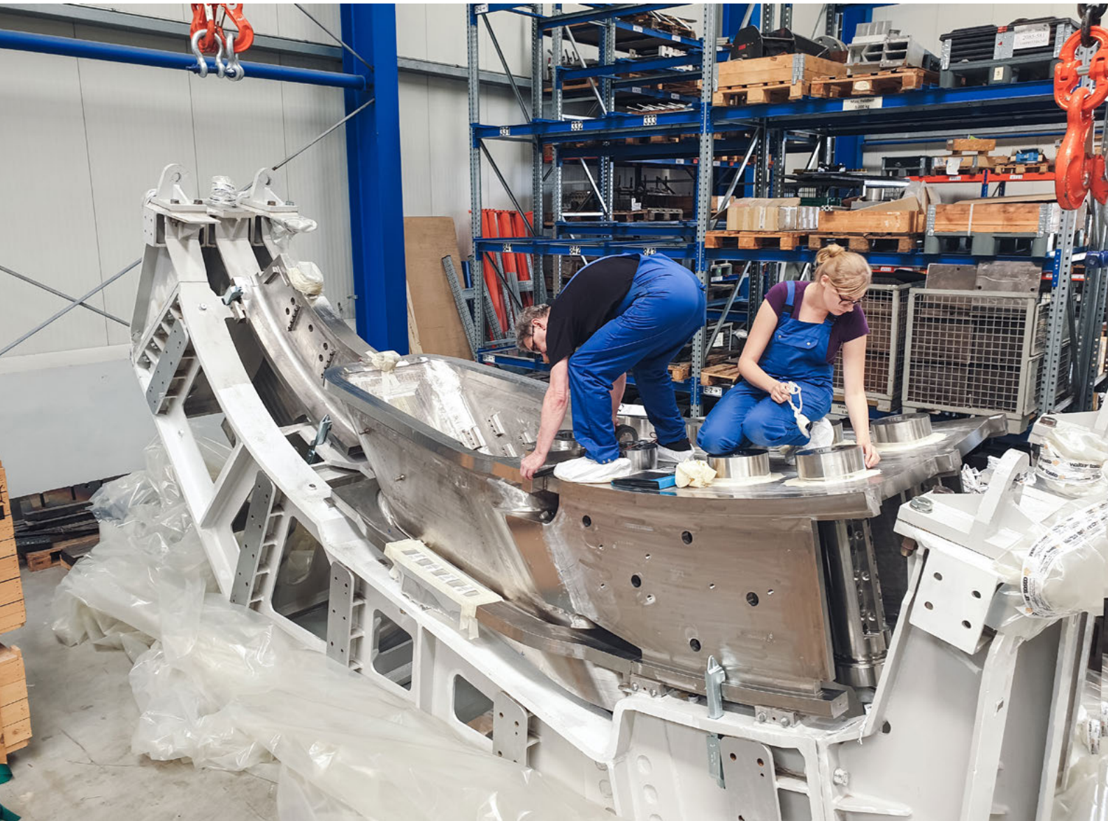
Before welding: Inspection at ProBeam of the last sector 5 assembly with a central port arriving from Walter Tosto.
