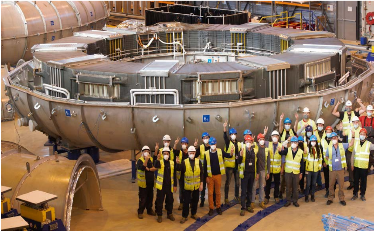
Figure 9: Poloidal Field Coil #6 completed and fully tested in Cadarache.
