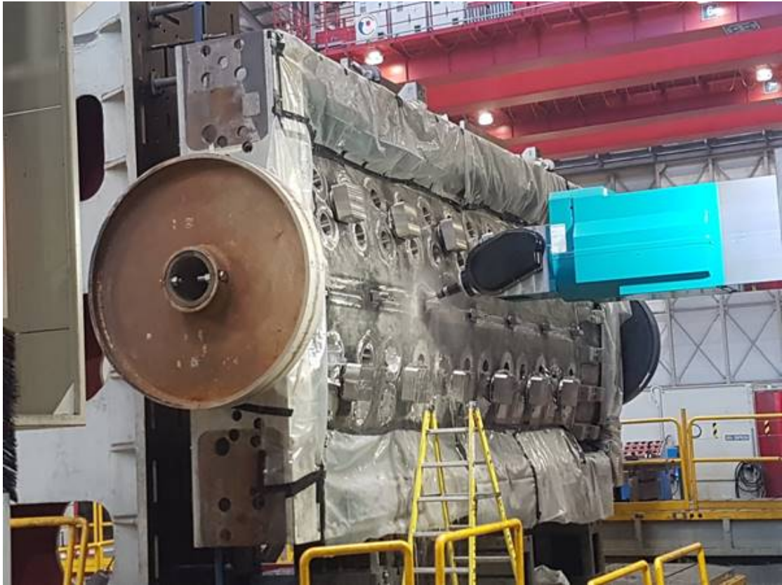
Figure 6: Machining of Sector 5 PS1
