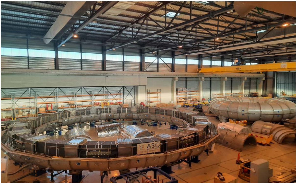
Figure 10: Poloidal Field Coil #5 ready for final Cold Test.
