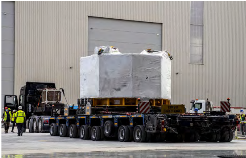
First central solenoid module, a 1 200-tonne magnet coil, arrived in September at the ITER site, France. The second module arrived towards the end of October. © ITER Organization
