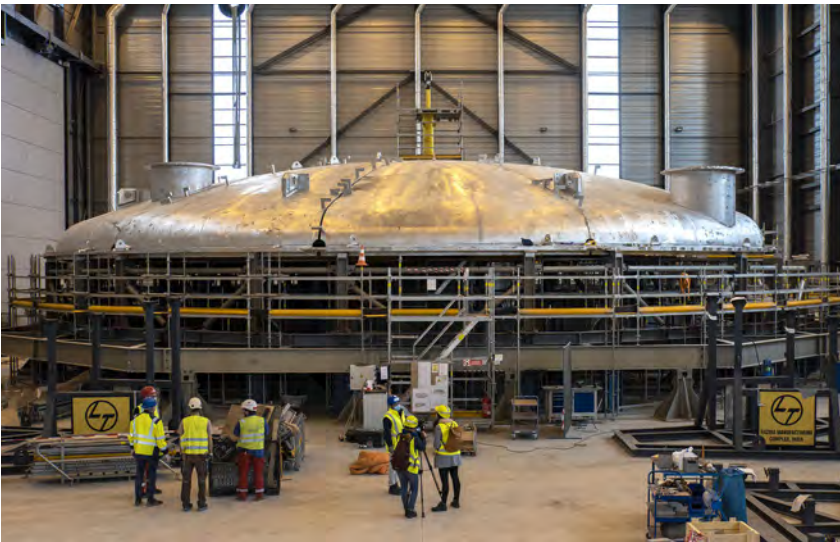
Seven of the 12 segments of the cryostat's top lid have been assembled on the work platform. March 2021 © ITER Organization
