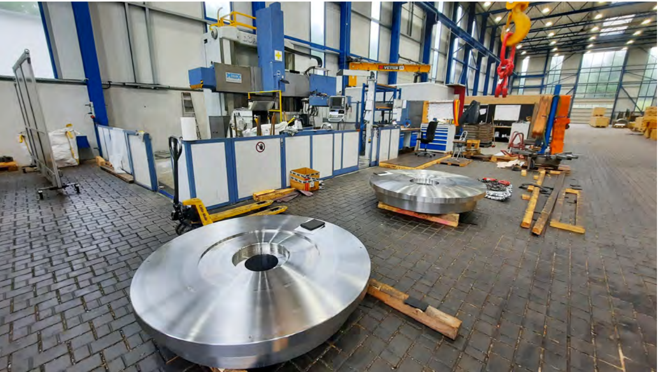
Two pump plugs in the workshop, not yet fully machined. These are the biggest components of the cryopumps. France, July 2021. © ALSYOM
