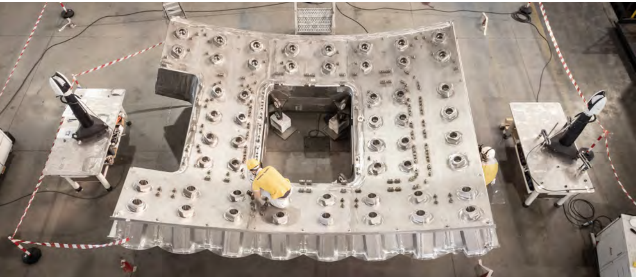
Technicians performing dimensional checks on Europe's vacuum vessel sector 4, poloidal segment 3, Walter Tosto, Italy, December 2021. © Walter Tosto
