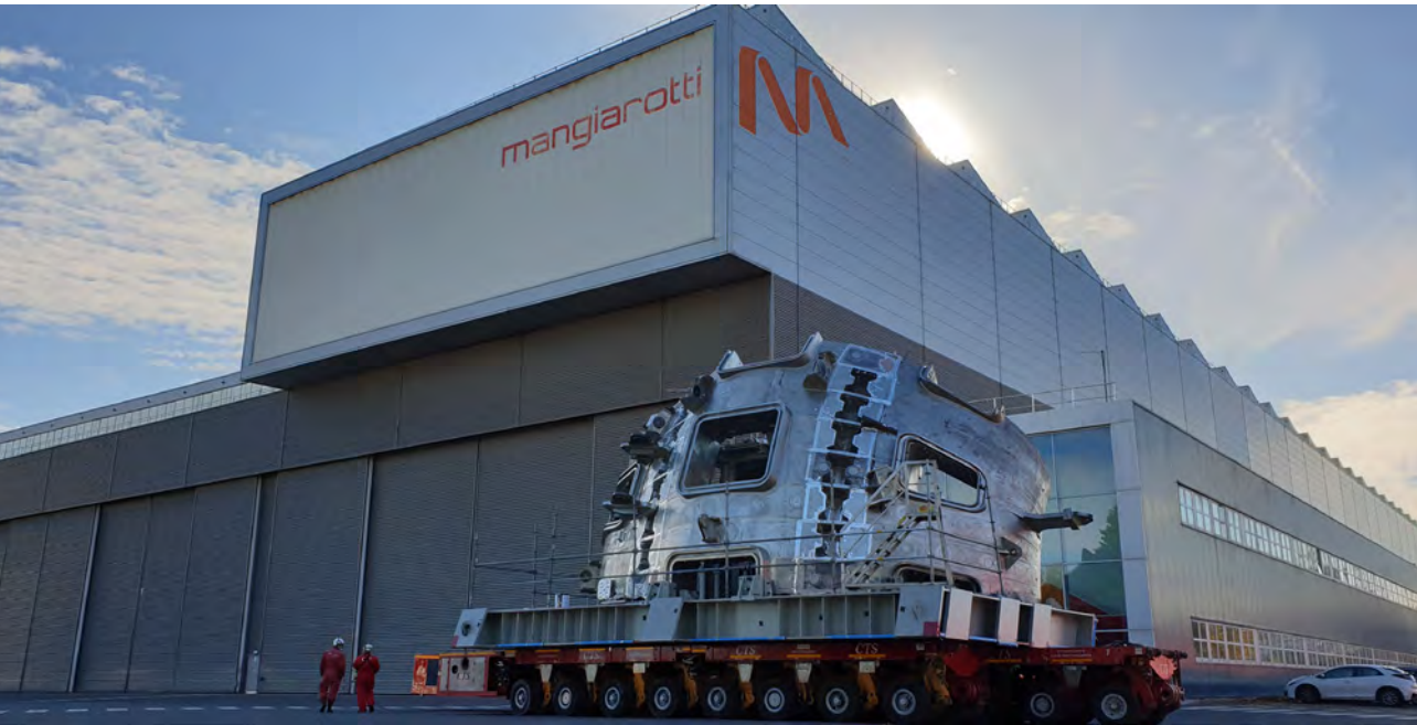
Europe's vacuum vessel sector 5 leaving the radiographic bunker of Mangiarotti to go through final tests, Mangiarotti, Italy, November 2021. © Mangiarotti
