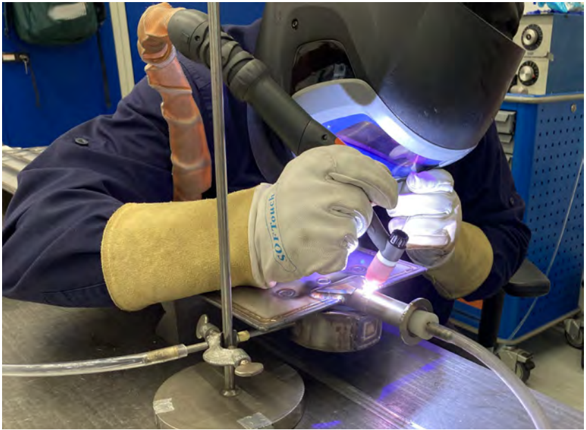
Welding the cryopanel at Research Instruments (RI), Germany, August 2021. These rectangular-shaped components measuring 1 m long and 0.2 m wide will perform the pumping by trapping the gas particles in their supercold surface. © RI
