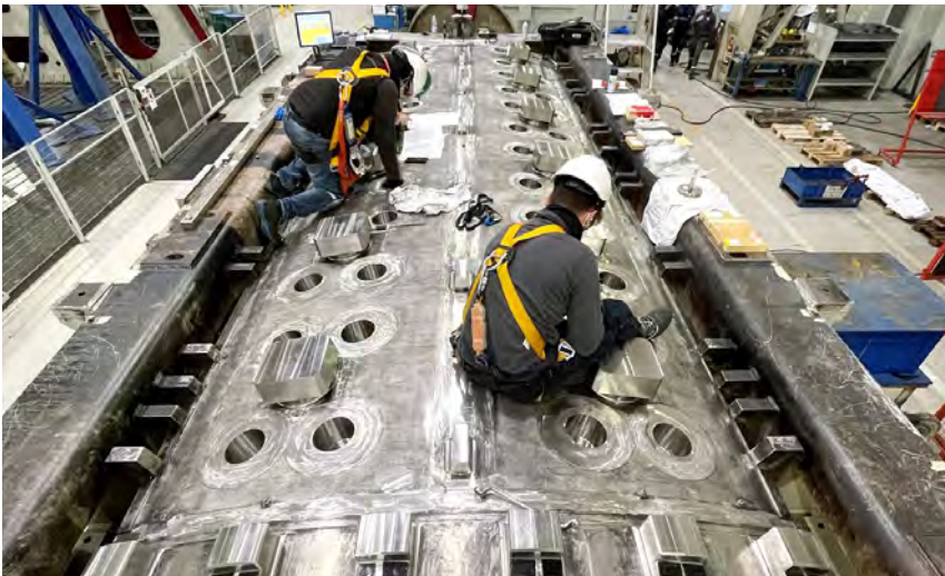
Inspector checking vacuum vessel sector 3, poloidal segment 2 at Walter Tosto, Italy, April 2021 © F4E
