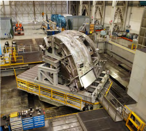
Placing on the jig in the factory of Mangiarotti, poloidal segment 4, manufactured by Mangiarotti, Italy, June 2021. The component is part of sector 5 of the ITER Vacuum Vessel manufactured in Europe. © F4E
