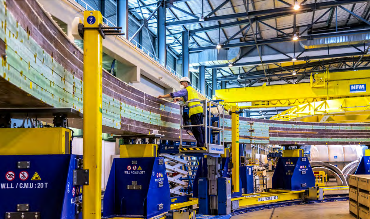
ITER Poloidal Field coil 4 in fabrication. Technician checking the stacking of the Double Pancakes of the magnet, which measures 24 m in diameter. Manufacturing performed in PF coils factory, Cadarache, France, December 2021. © F4E
