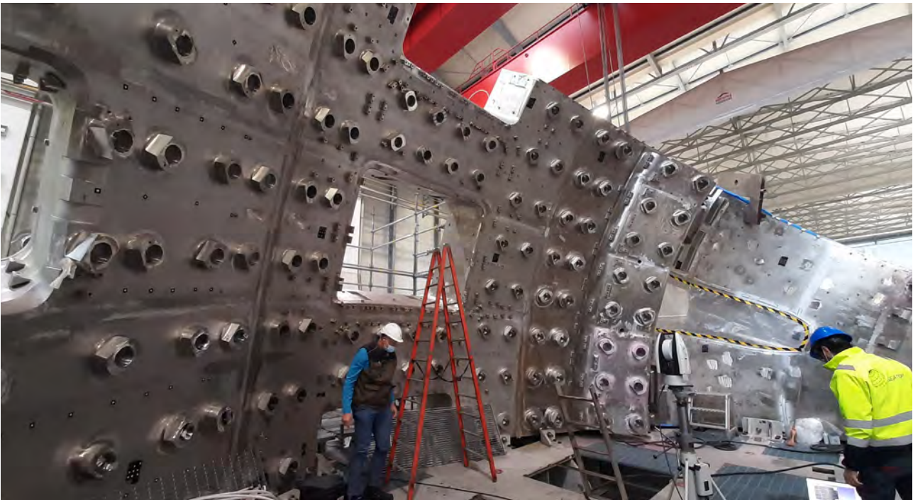
A part of ITER Vacuum Vessel sector 5, holed like a Gruyère cheese, with dozens of housings. Mangiarotti, Italy, November 2021. © F4E
