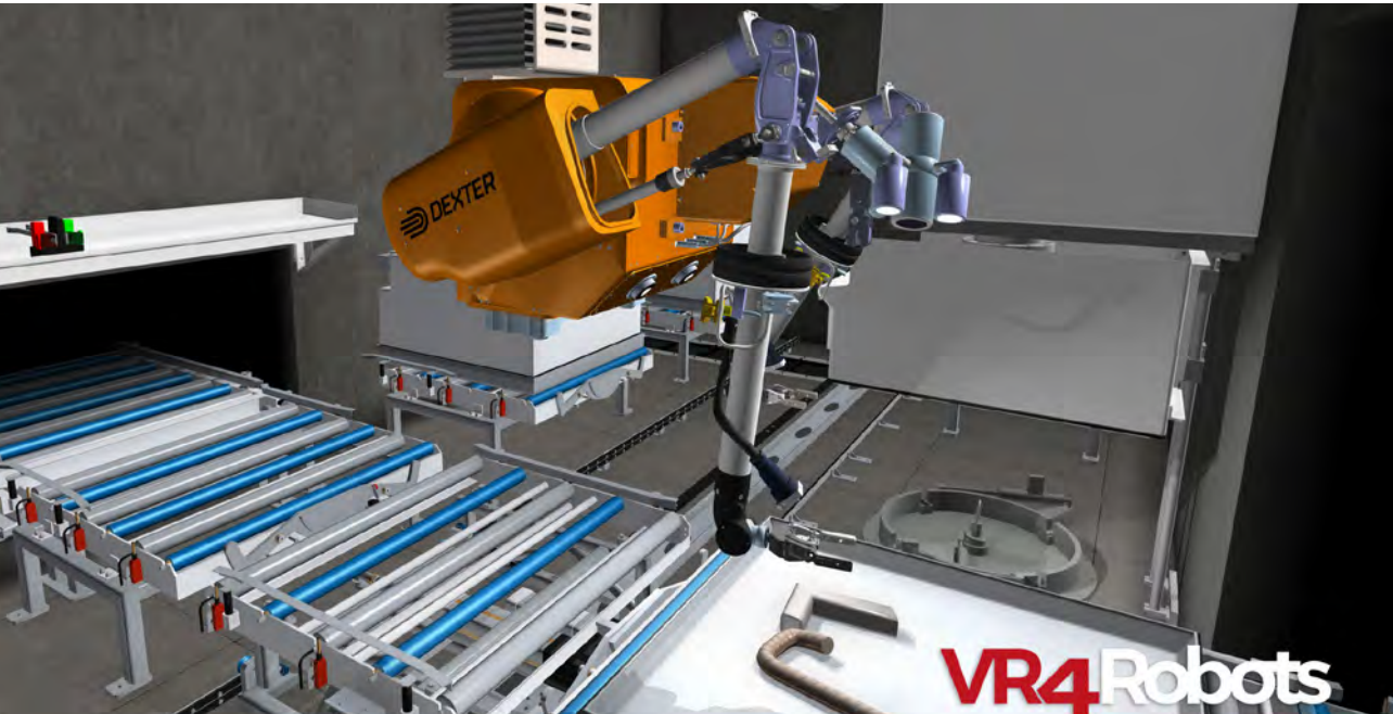
Retiina remote handling simulator; a VR4Robots physics-based digital twin of Veolia Nuclear Solutions' Dexter Remote Manipulator System. © Veolia Nuclear Solutions (UK) & Tree C Technology
