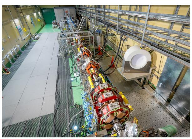
SPD\_figure 10 . IFMIF/EVEDA - View of LIPAc (Linear IFMIF Prototype Accelerator) in the complete phase B+ configuration to demonstrate operation with a deuterium beam of 125 mA at 5 MeV in continuous operation during at least 30 minutes
