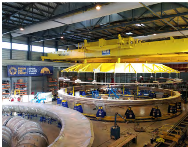
Stacking of the final Double Pancake of ITER Poloidal Field coil 3, performed in Europe's PF coils factory, Cadarache, France, December 2022. ©F4E
