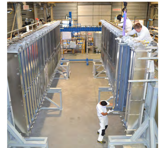
Operators placing a pumping section in the MITICA (Megavolt ITER Injector and Concept Advancement) Cryopump, France, October 2022. ©SDM
