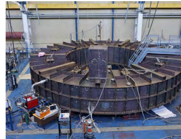
Sredne-Nevisky Shipyard (SNSZ) specialists have successfully finished factory acceptance tests on poloidal field coil #1 (PF1) in Russia. March 2022. ©ITER Organization
