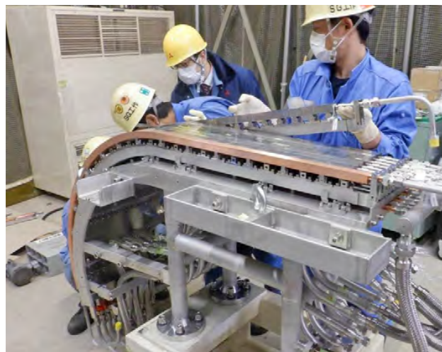
Plasma-facing units of the ITER divertor outer vertical target prototype have been mounted on a test assembly for high heat flux heating in Japan. January 2022. ©ITER Organization
