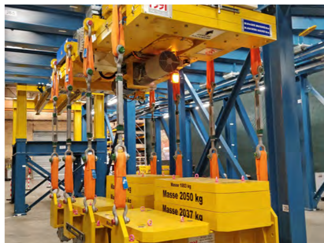
The neutral beam remote handling crane prototype in REEL's premises, France. May 2022. ©F4E
