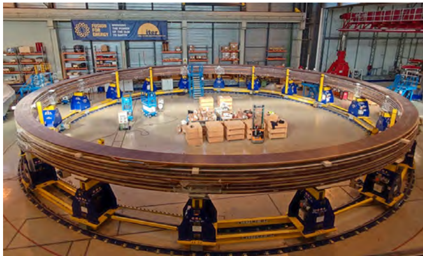
Figure 9: PF Coil #3 Winding Pack stacking completed at the PF Coils Workshop
