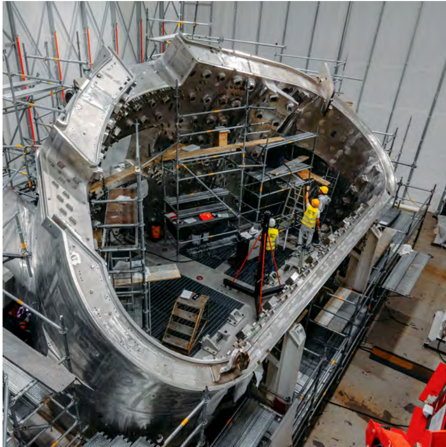
Figure 6: Sector 5 in Sector Assembly phase at Mangiarotti
