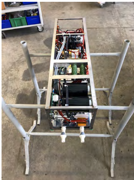
Figure 32: Manufacturing of the first Power Module for the Residual Ion Dump Power Supply of ITER
