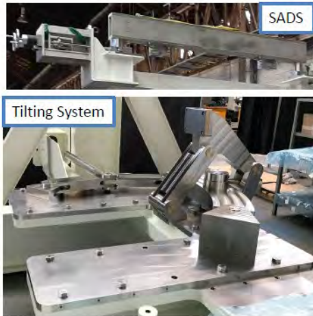
Figure 26: The main sub-assemblies of the MITICA Beam Source completed in 2022 (MUBS: Mock-Up of the Beam Source, BSHT: Beam Source Handling Tool, MUIS; Mock-Up of the Installation, TS: Tilting System, SADS: Supporting and Adjustment System)
