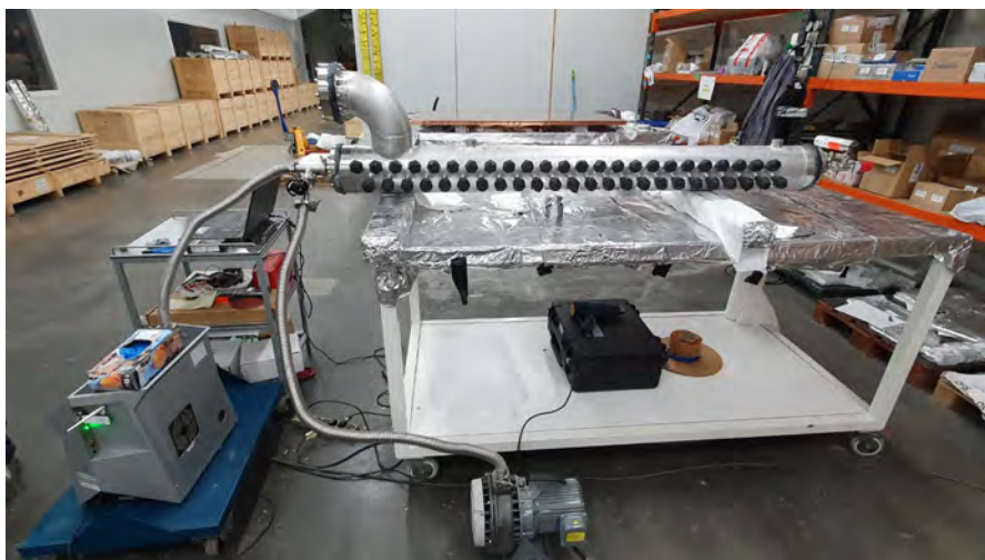
Figure 28: A manifold of the Calorimeter undergoing a leak test after welding NBTF auxiliary systems
