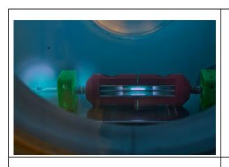
JT-60SA - F4E Cold Cathode Vacuum Gage – Under calibration
