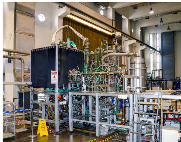
The ITER India Gyrotron Test Facility successfully completed the site acceptance of a test gyrotron for ITER power and pulse requirements, including all the associated auxiliaries. March 2023. ©ITER Organization
