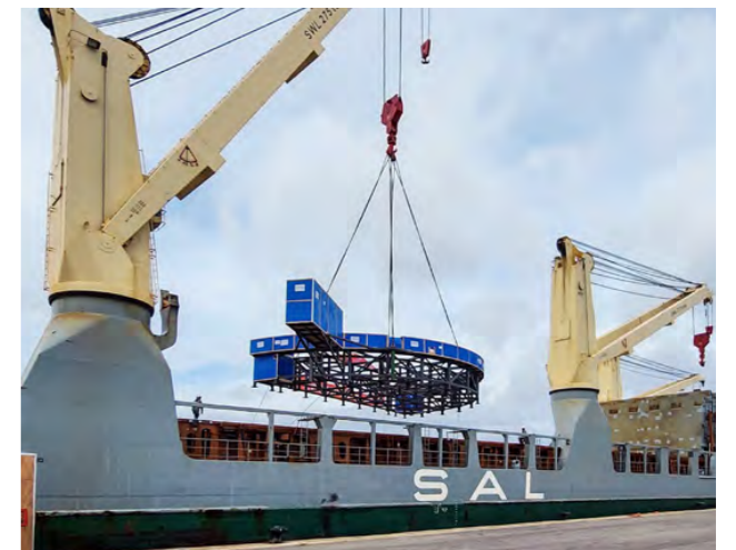
The in-cryostat feeder left from China and arrived in France. This semi-circular component will fit inside the cylindrical cryostat to deliver power, cryogens and instrumentation to four of the top correction coils. October 2023. ©ITER Organization
