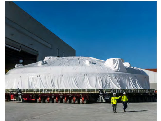
The 665-tonne cryostat top lid is stored under protective wrap. April 2023. ©ITER Organization
