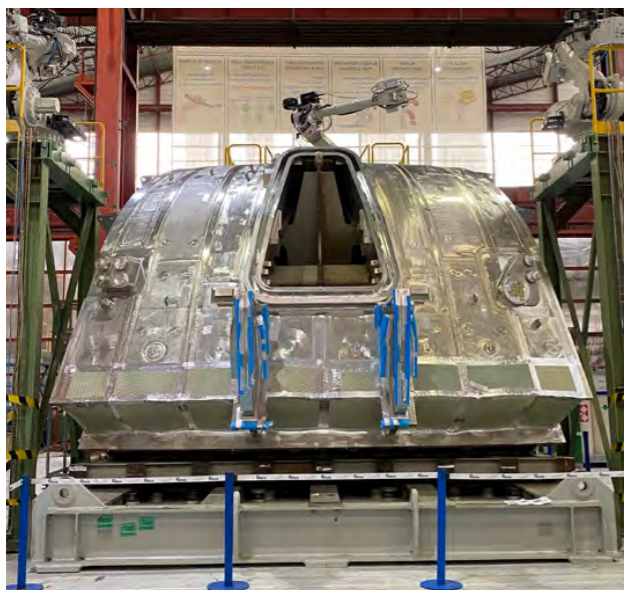
One of Europe's segments (PS4 of Sector 2) where ENSA performed welding operations with the help of robots, ENSA, Spain, March 2023 © ENSA
