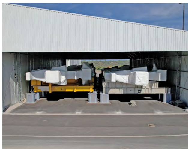
Two toroidal field coils rest on their sides in storage. They will be called back into the Assembly Hall when works with other components advance. October 2023. ©ITER Organization
