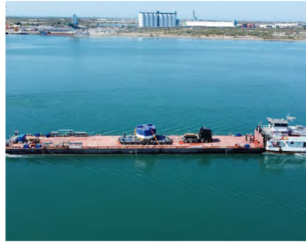
Like the solenoid module in the picture, some of the bigger components arriving at the port of Fos-sur-Mer then cross the inland sea of Barre on a barge on their way to ITER. July 2023. ©ITER Organization
