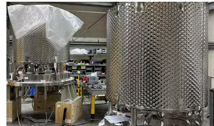
Two of the torus and cryostat cryopumps during the factory acceptance tests at Research Instruments. November 2023 ©RI
