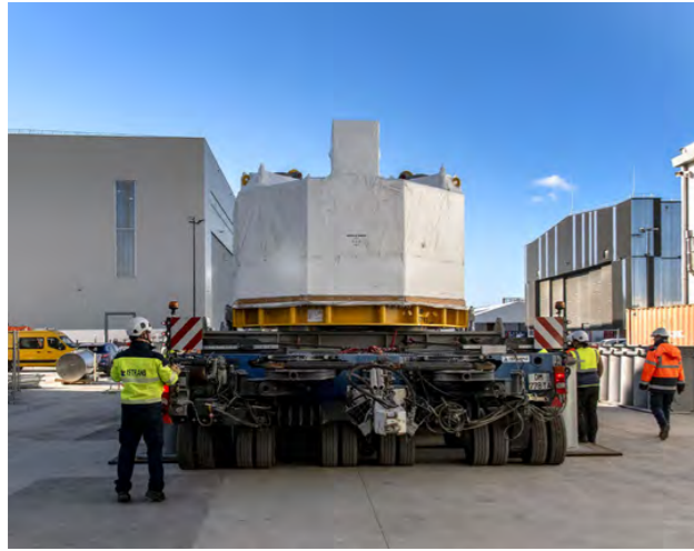
US ITER and its contractor General Atomics delivered the third and fourth out of seven central solenoid modules, each weighing 110 tonnes and standing 2 metres high. December 2023. ©ITER Organization
