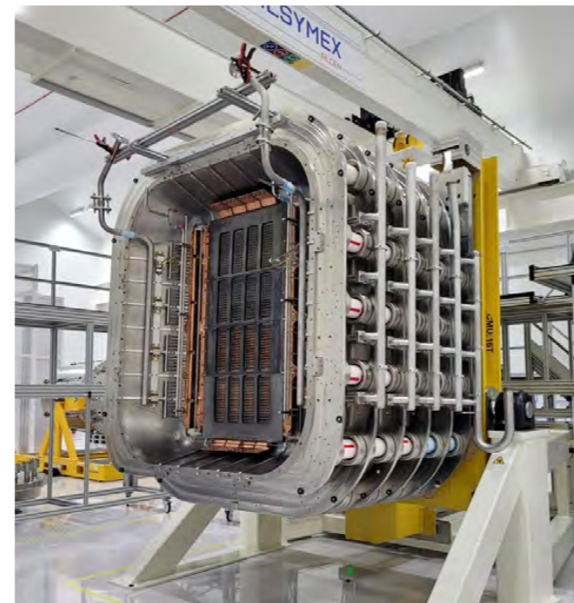
The five stages accelerator of the MITICA beam source fully assembled together with the extractor. November 2023 ©Alsymbex
