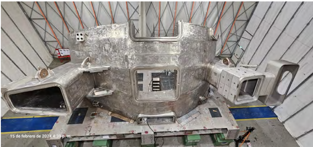
Figure 7: Sector 5 After declaration of conformity of all 2598 welds at Mangiarotti
