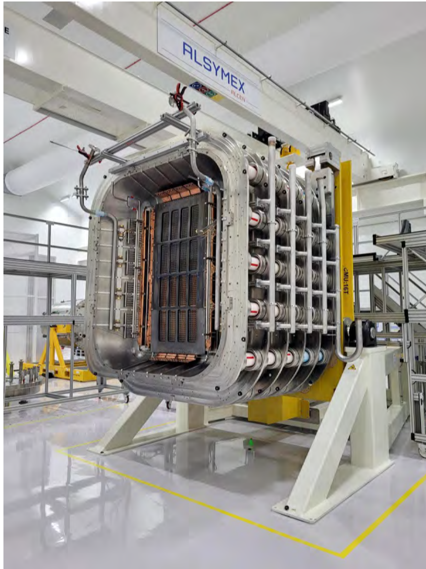
Figure 25: The five stages accelerator of the MITICA BS fully assembled together with the extractor.
