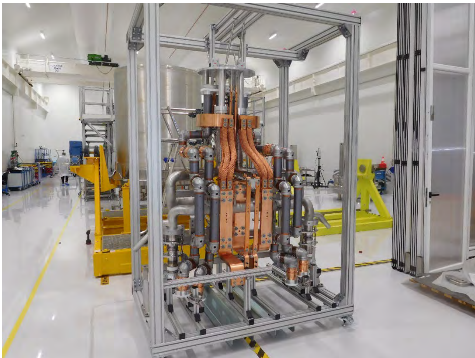
Figure 26: The Top Flexible Connection of the MITICA BS in the assembly structure.
