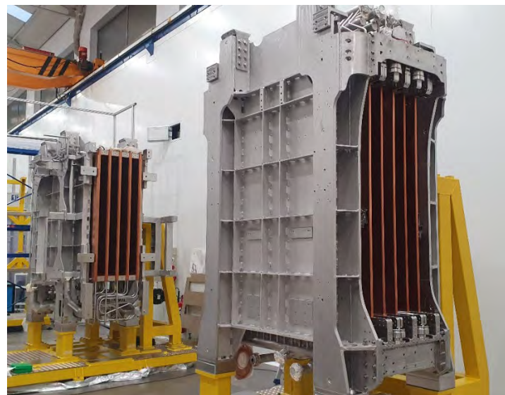
Figure 28: On the right the Residual Ion Dump with the panels mounted on the support structure and the stand-off insulators mounted. On the left the Neutralizer with the sandwich of panels assembled and pipe work completed.
