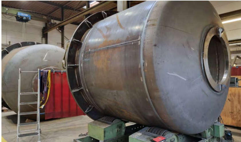
Figure 32: Connecting Box Vessels of the High Voltage Bushing Assemblies under manufacturing.
