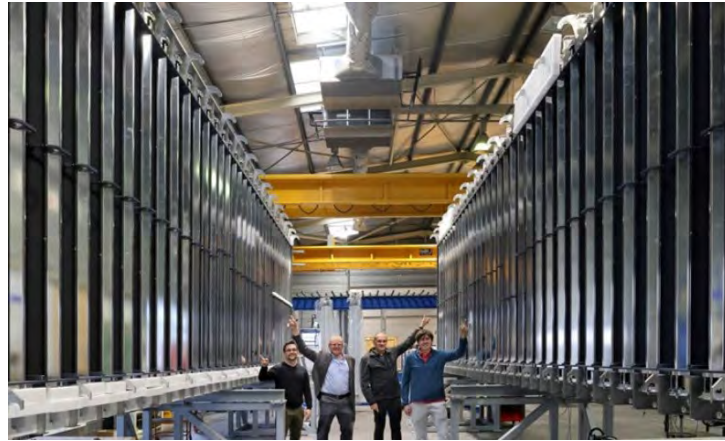
Figure 21: MITICA cryopumps ready to be delivered.
