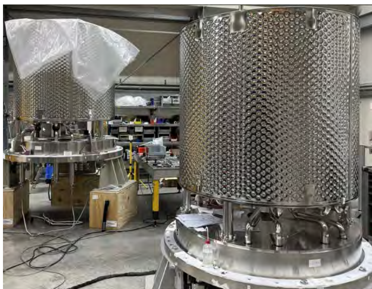
Figure 24: Ongoing Torus and Cryostat Cryopump assembly.
