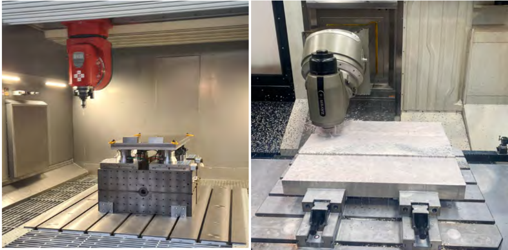
Figure 12: Pre-Series First Wall panels under manufacturing at FBL (Spain) and Alsymex (France) workshops.
