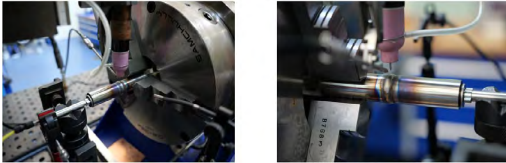
Figure 17: Qualification of dissimilar weld joints between EUROFER97 and stainless steel SS316L(N)-IG, pipe GTAW welding (CEA credit).
