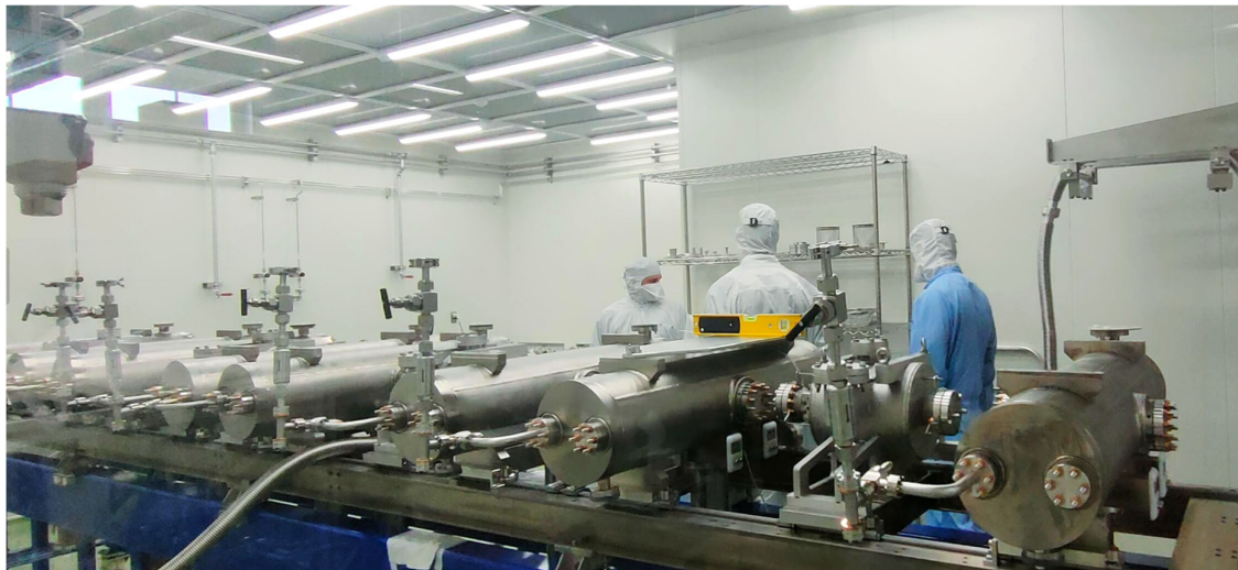
SPD_figure 12 . Assembly activities in April 2024 in the clean room on the Rokkasho site. The superconducting cavities mounted on their support frame are visible in the foreground.
