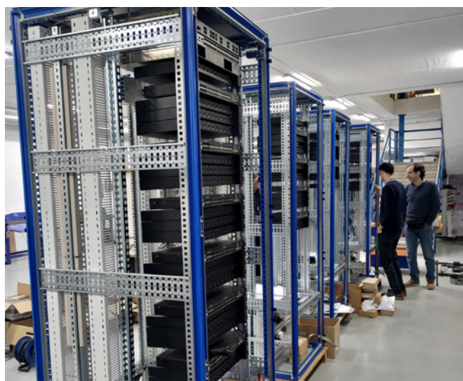
F4E colleagues revise the electronic cabinets during assembly with the electronics (black boxes) already installed. October 2024. ©F4E
