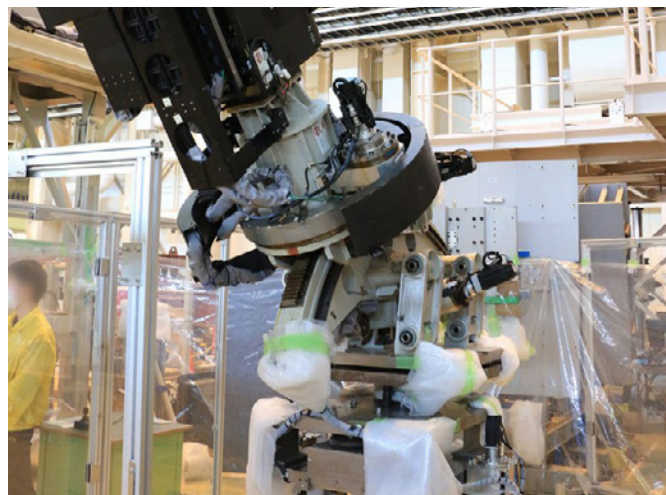
A robotic manipulator arm, part of the remote handling system to replace first wall panels, undergoing testing. June 2024. ©ITER Organization
