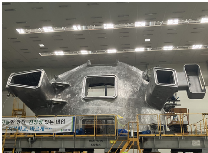
Korea's fourth and last ITER Vacuum Vessel sector completed and ready to leave the factory of Hyundai Heavy Industries. 2024. ©ITER Korea
