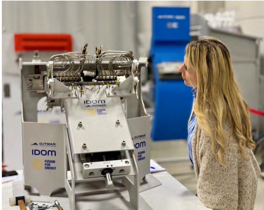
Figure 32: Prototype of the in-divertor electrical connector, developed by IDOM and GUTMAR to simulate and verify the challenging engagement and disengagement operations each time the divertor cassette is replaced.
