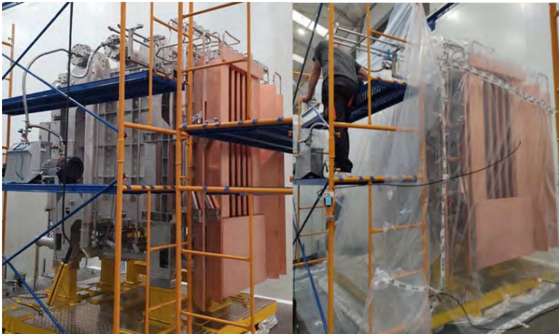
Figure 38: Neutralizer FAT milestone successfully passed- Neutralizer during FAT leak testing.
