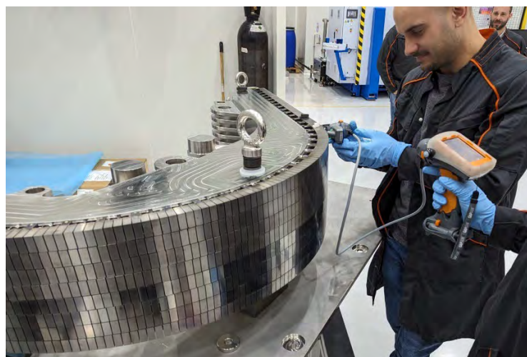
Figure 58: Dimensional Inspection of IVT Gap/Steps.
