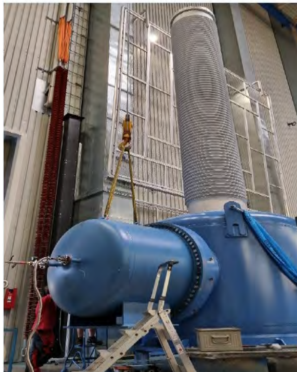
Figure 40: Successful leakage tests of the HV Bushing Assembly.
