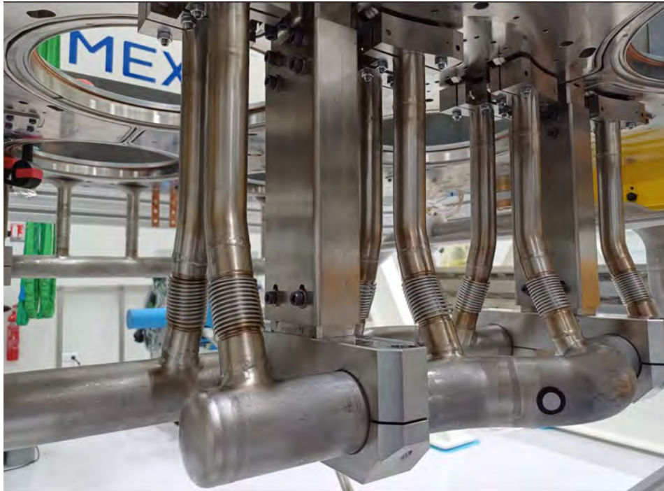
Figure 36: PDP central pipes group welded with replaced bellows.
