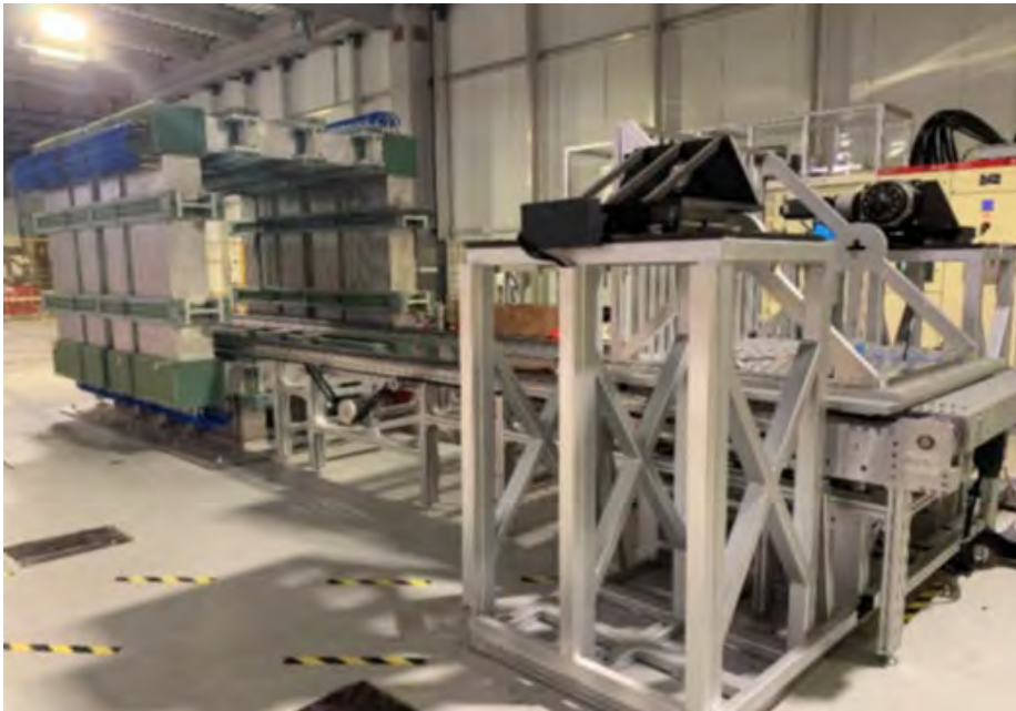
Figure 27: Static magnetic field test facility and instrument arrangement on test rig.
