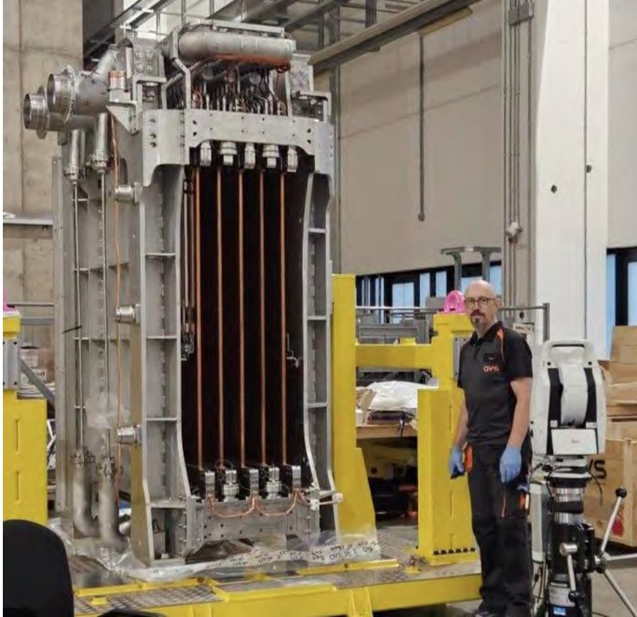
Figure 37: The Electrostatic Residual Ion Dump (ERID) dimensional inspection at MITICA facility.
