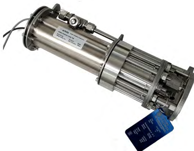
Figure 34: Prototype, produced by ARKTIS for ENEA, of the RNC ex-vessel neutron detector which uses high-pressure He4 as a scintillator.
