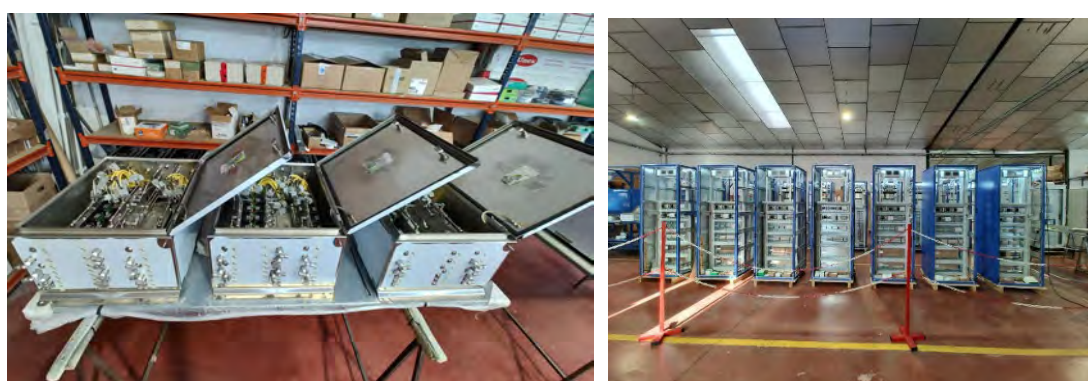
Figure 67: Manufacture of 14 x Control Cubicles (LCCs) and 17 x Pneumatic Enclosures (WMEEn) for Cold Valve Boxes and Cyopumps I&C
