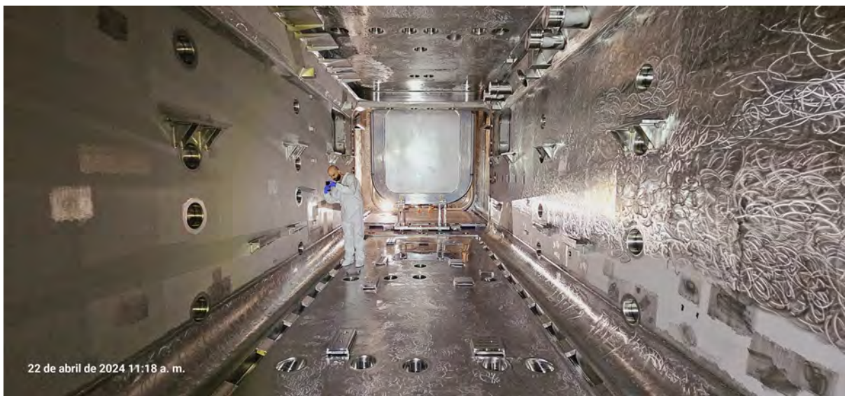
Figure 60: Dimensional Inspection of MITICA Vessel.
