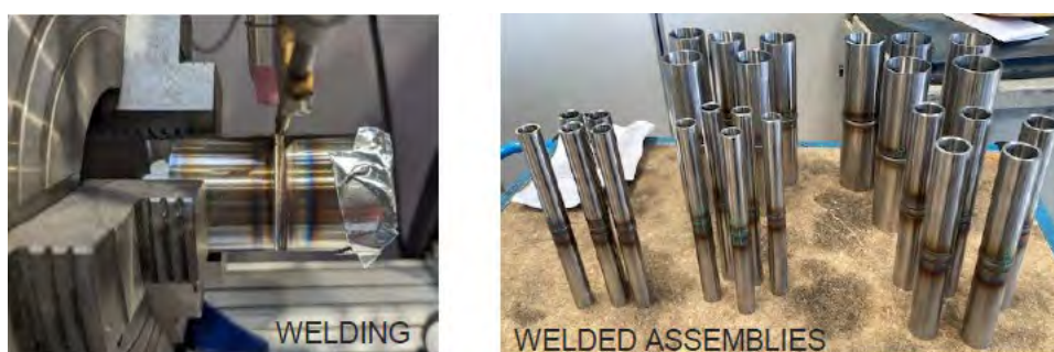
Figure 15: Qualification of dissimilar weld joints between EUROFER97 and stainless steel SS316L(N)-IG, pipe GTAW welding (CEA credit).
