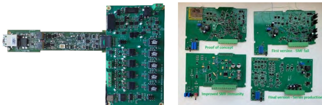
Figure 66: Left, bolometers driver & DAQ functional prototype developed by F4E. Right, Development of a SIL3 signal conditioner for the Hydrogen Monitoring System.
