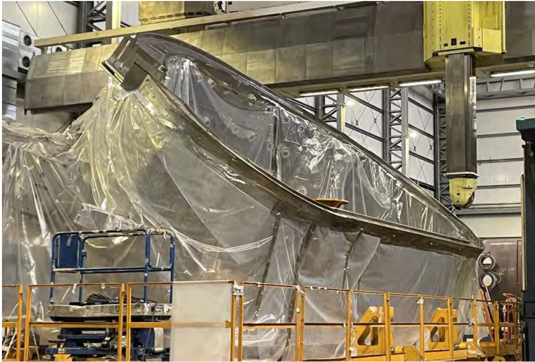
Figure 7: Sector 4 under final machining of Field Joints at WTO
