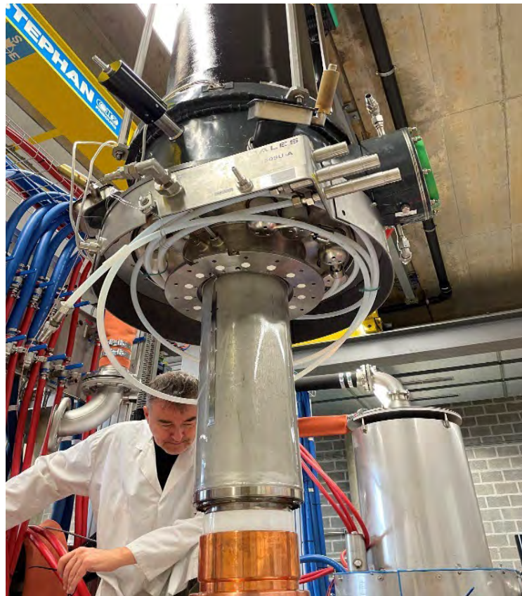
Figure 44: DTT pre-series gyrotron was successfully tested at the F4E FALCON facility in 2024
