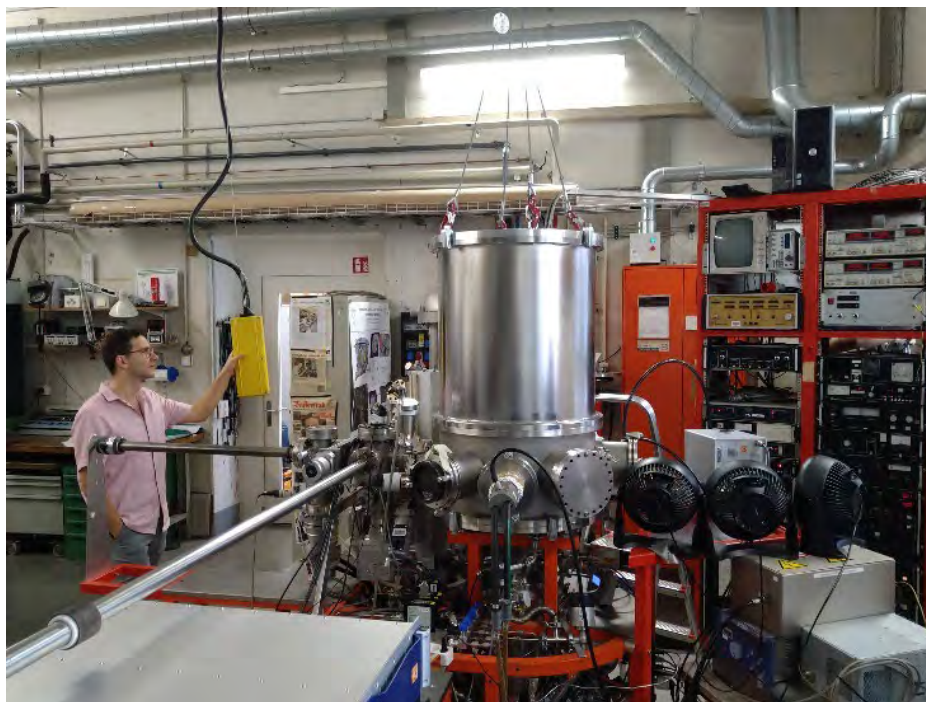
Figure 29: Facility at University of Basel used to demonstrate the use of radio-frequency plasmas for in-situ cleaning of the large, CPTS plasma-facing mirror.
