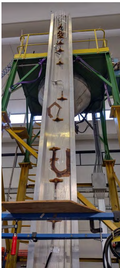
Figure 46 - The 1:1 scale mock-up of the central solenoid used to validate the repair procedure
