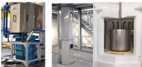
Figure 63: The KALOS-UP facility (KIT) is the only European facility to produce ceramic breeder pebbles
