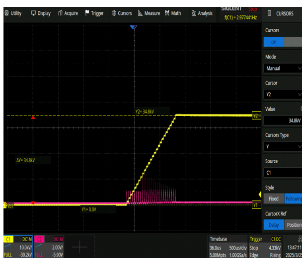
Figure 42: March 2025 High Voltage Body Power Supply (HV-BPS) Commissioning 35kV output achieved
