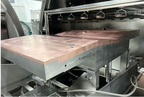
Figure 7: Pre-Series Panels at Alsymex during Hot Helium Leak Tests
