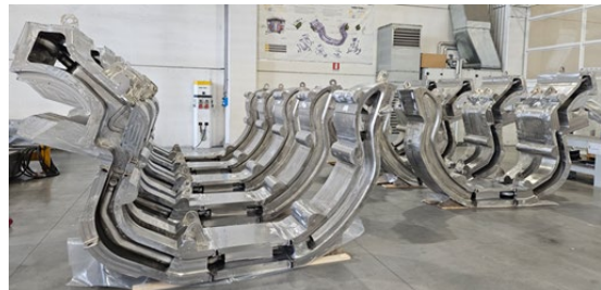
Figure 14: CBS structures under fabrication at Walter Tosto premises
