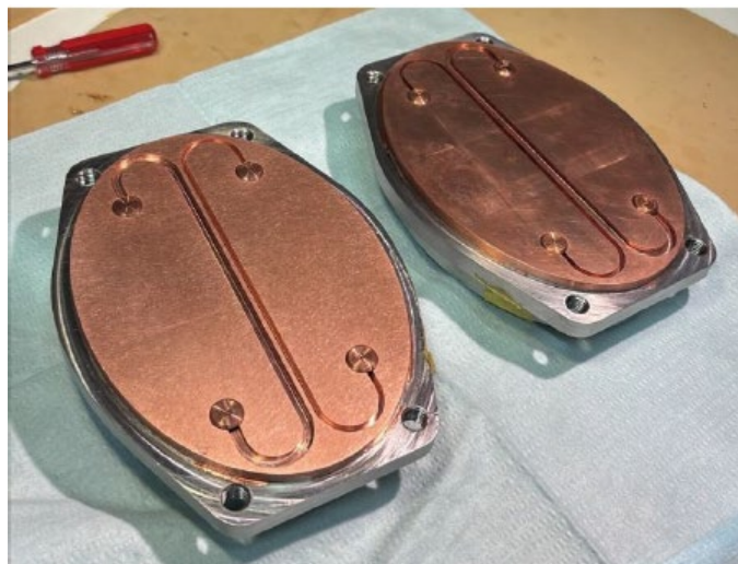
Figure 56: Copper electrodeposition on launcher mirrors for CTS
