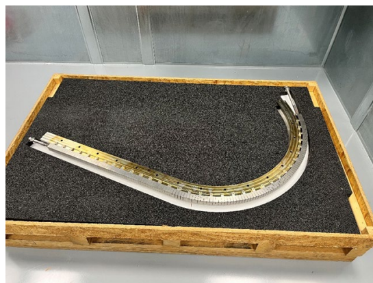
Figure 19: First Plasma facing Unit successfully tested
