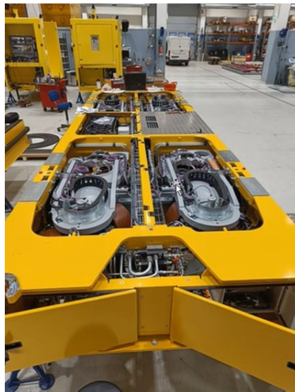
Figure 26: CTS under final assembly prior to initial testing with the Ansaldo sub-contractor
