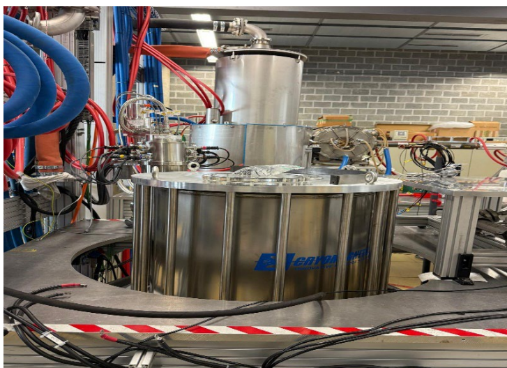
Figure 45: New magnet by Cryomagnetics and DTT pre-series gyrotron at FALCON September 2025
