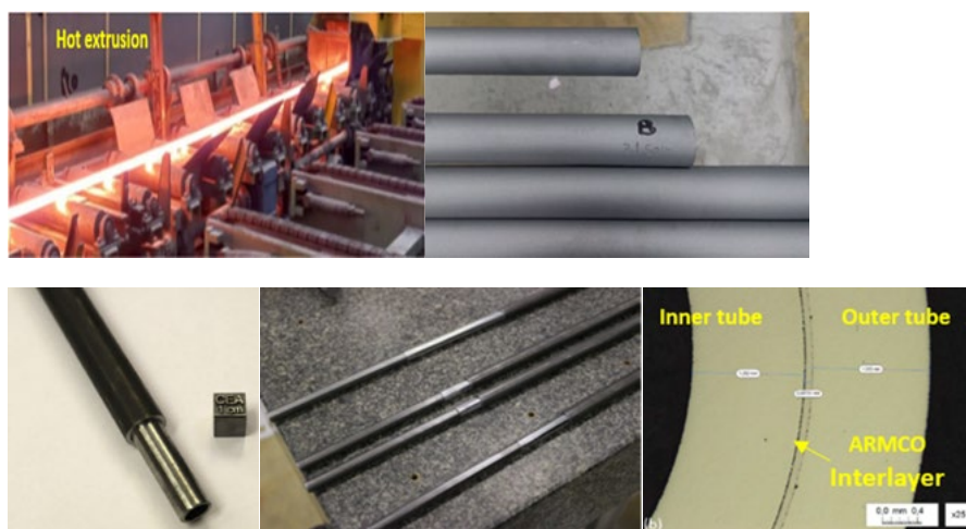
Figure 60:Manufactured EUROFER97 double-wall tubes (DWTs), including representative macrographs
