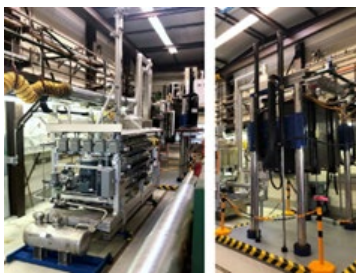
Figure 61: MaPLE (KIT) uses prototypical eutectic PbLi (MP: 235 °C) at 300°C and enables experiments with combined MHD and buoyancy effects
