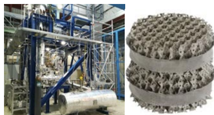
Figure 64: GLC characterization in TRIEX-II (ENEA) for tritium extraction
