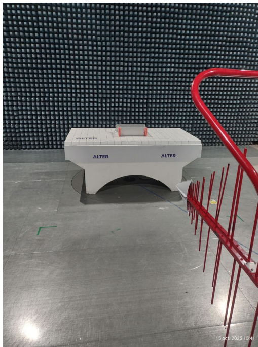
Figure 54: Test setup of Bolometer electronics in a semi-anechoic chamber
