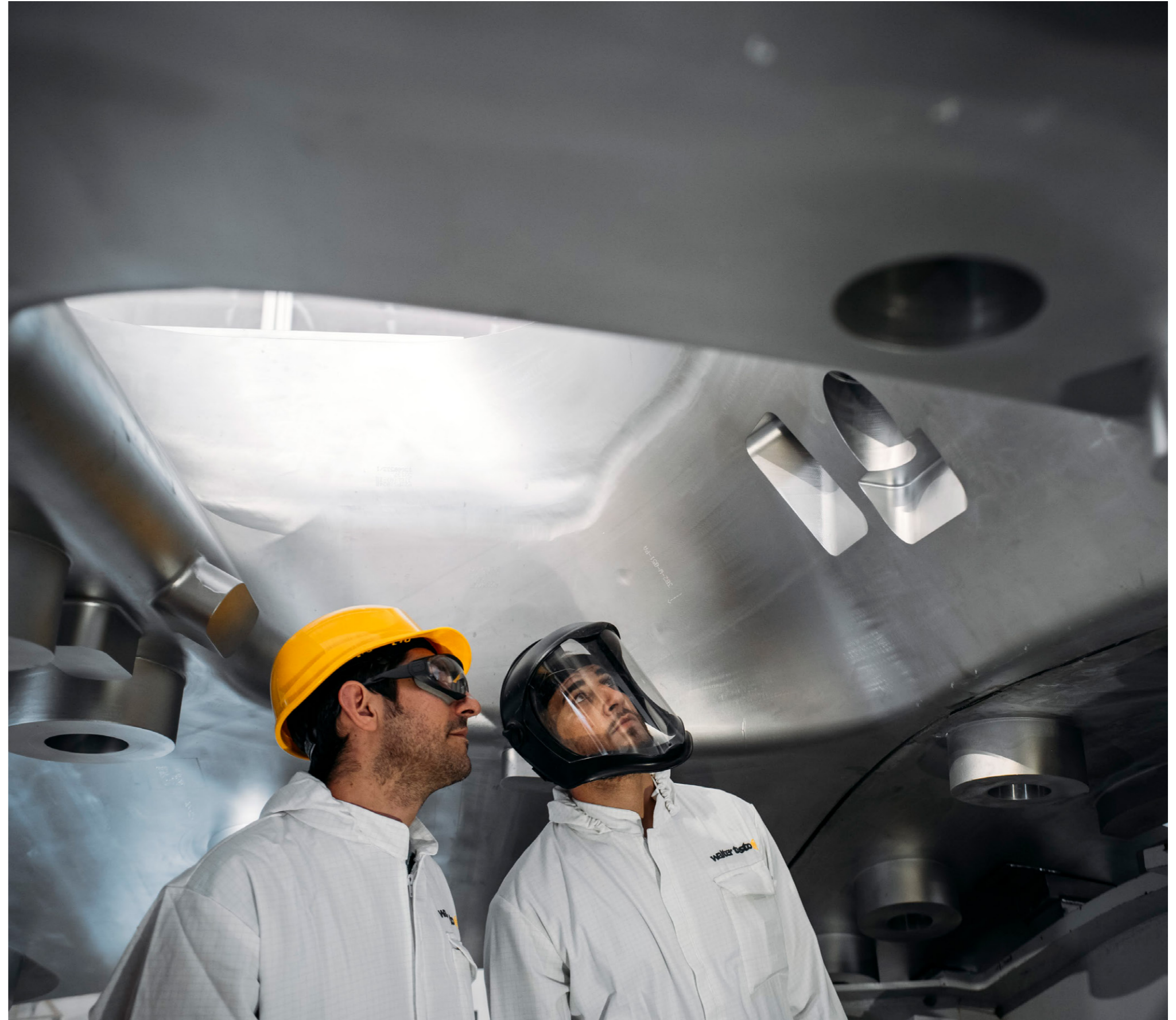
Technicians of Walter Tosto inspect an ITER Vacuum Vessel sector during manufacturing. ©F4E
